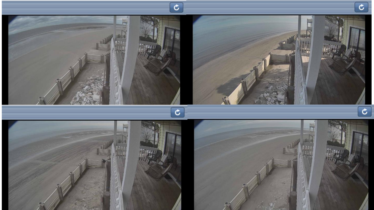
Figure 31. Typical trench self-healing and accretion over a three day period (January 25-January 27, 2016). Note bags being covered by accreting sand.
